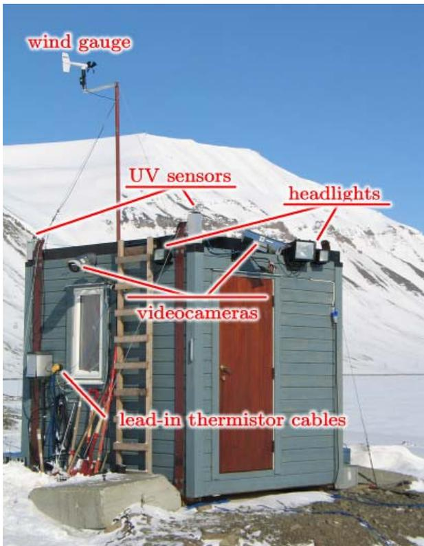
Figure 8. Weather station and instrumentation hut (September 2006).
