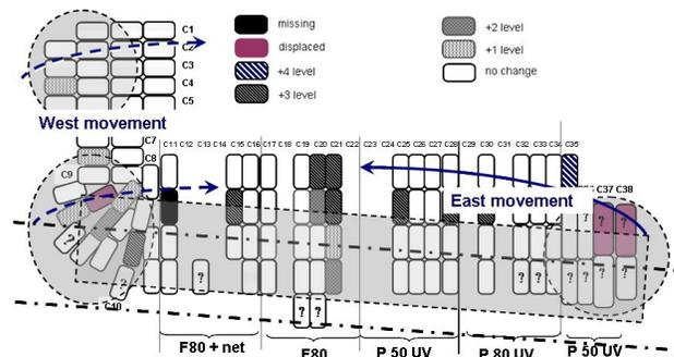
Figure 16. Evolution of the damages observed on the bags during 1 year (summer 2008 to summer 2009) in relation with the different ice actions either from East or from West.)
