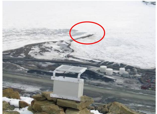
Figure 9. Time lapse camera on Liljevalchfjellet above Svea taking pictures of the sea ice in Sveasundet, May 22nd 2007. The experimental breakwater in the red circle (Caline, 2010)
