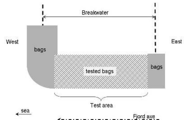
Figure 2. Design of test bags location.
