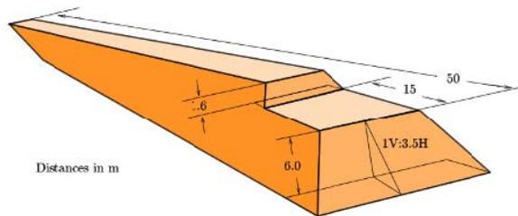
Figure 4. Sketch of the breakwater (Caline, 2010).
