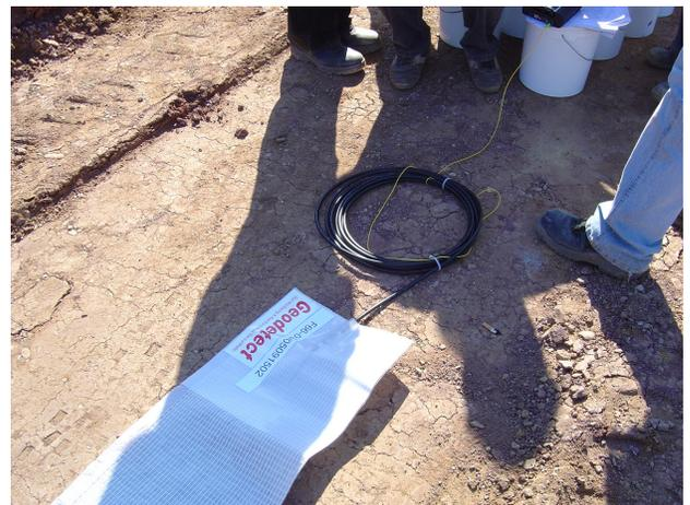
Figure 11. The TenCate GeoDetect® textile fiber optics sensor
