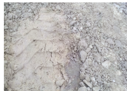
Test section using a 4 oz nonwoven geotextile and a multi-axial geogrid with 3' minus basalt stone. Picture shows the 3" stone ruptured the multi-axial grid after the first few passes.
