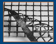
Miragrid® XT High strength reinforcement geogrid comprised of high tenacity polyester fibers coated with a polymer coating.
