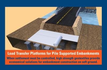
TenCate Mirafi® geosynthetics (i.e., geogrids and geotextiles) MSE system solutions cost significantly less than conventional structures, and the rapid, simple installation process greatly shortens construction schedules. Their flexibility allows them to be used in both large industrial and small residential applications, with a proven performance in walls, slopes, and embankments.
