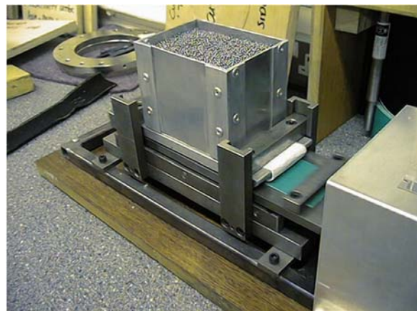
Figure 7: ENV ISO 10722 - Procedure for simulating damage during installation
