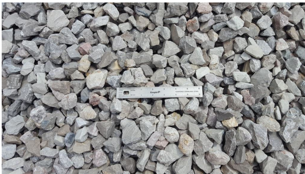
Figure 4-2. Installation damage Type 1 test aggregate.
