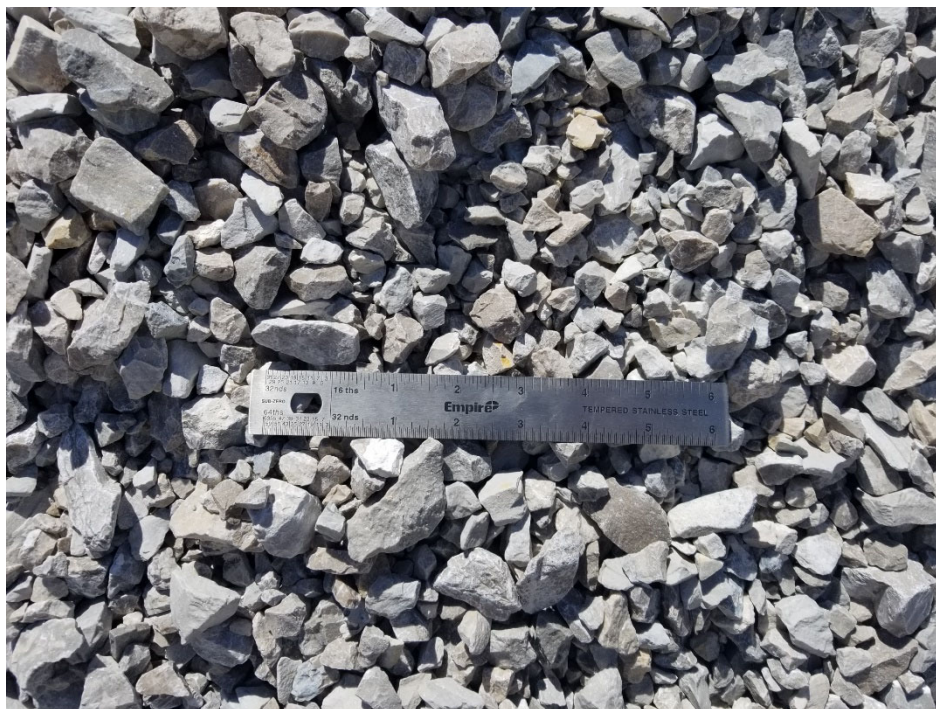
Figure 4-4. Installation damage 57 stone test aggregate.
