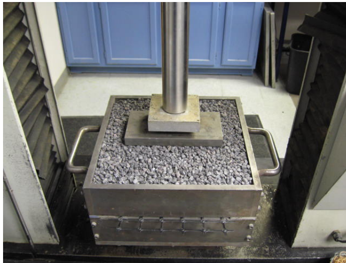
Figure E-1. ISO/EN 10722, laboratory installation damage test apparatus.
