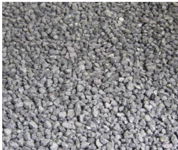
Figure E-2. ISO/EN 10722, laboratory installation damage aggregate.
