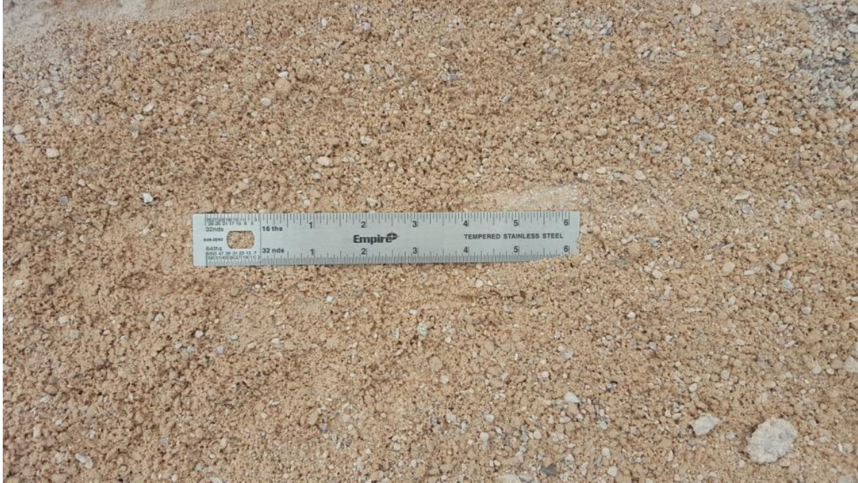
Figure 4-5. Installation damage Type 3 test aggregate.
